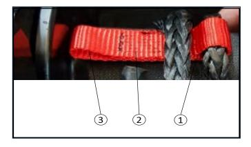
Winch Rope tail inserted through second loop of the Plasma Lock(**3**).
