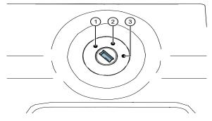
Apply pressure to the foot brake, turn the key to position (3) until engine starts. Once the engine has started, release the key. This will allow the key to rotate back to position (2).
