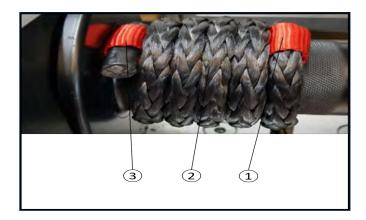
The following image shows the Plasma Lock fully engaged with the Winch Rope inserted **(1)**. You can see the Winch Rope wrapped around the Winch Drum and Plasma Lock four times **(2)** with the
