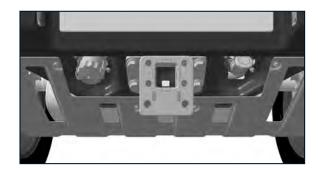
4. Insert the Removable Rear Winch into the 2" Receiver, ensuring the locking pin is correctly installed and secure with the R-Clip.
