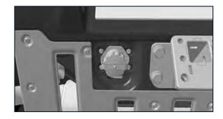
7. Inspect and remove any debris or material that may have been collected around the Winch Fairlead, before commencing any Winch operation.
