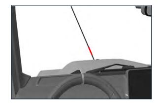
If you see either of the above, then the Winch Rope has reached its maximum extension length. The friction effect between the Winch Rope and Winch Drum will start to fail, if the Winch Rope is spooled out any further.
