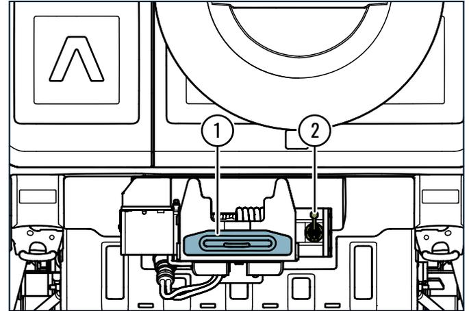
It has the same fixed components fairlead (1) and freespool lever (2) as the front winch except that it also has a locking pin for the square hitch receiver tube and a power cable that must be attached.
