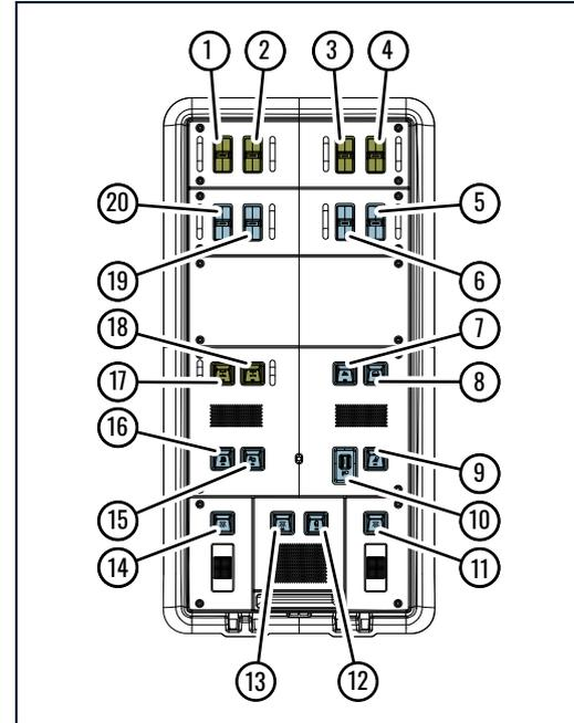
1. EXT 2: If equipped – Switch on or off 25A circuit A (front right roof outlet), of the exterior roof power outlets.
