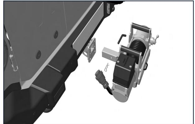
6. Inspect the Removable Rear Winch electrical cable for damage or wear.
