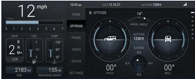
> TEMPERATURE shows tire, automatic transmission, and transfer case temperatures and tire pressure.
