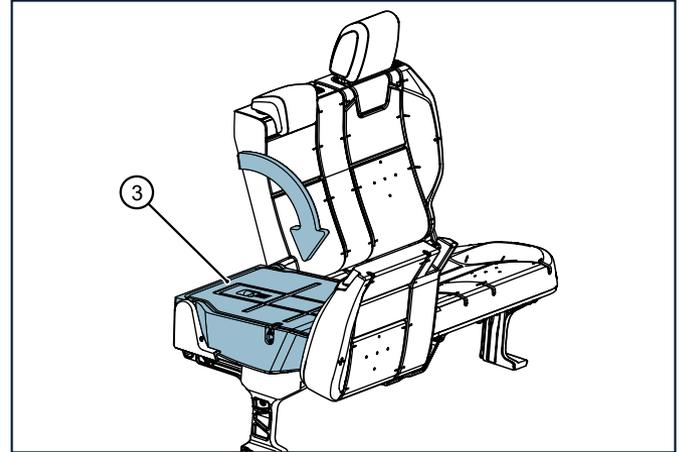
It is possible to fold the seat back forward to lie flat on top of the lower cushion without removing the head restraints. However, INEOS recommends removing the head restraint using the method shown above instead because it reduces the risk of contact between the head restraint and a front seat back or front seat occupant, and it protects the head restraint once that is stored away. Make sure to secure any head restraint that has been removed. Do not allow it to remain loose in your Grenadier.
