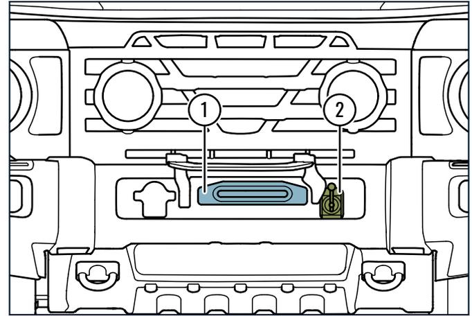
Its fixed components are a fairlead (1) which helps direct the winch rope onto the drum in a smooth and aligned manner. (The drum is behind the fairlead). The winch rope is stored on the drum and is routed through the fairlead for use. A freespool lever (2) activates a clutch. When it is vertical, the clutch is engaged, and the drum is held in place by the winch motor. When it is horizontal, the clutch is disengaged, and the winch rope can be pulled off of the drum.
