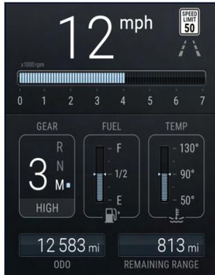
ISA can also detect electronic signs that are overhead or to the side of the road. ISA uses the map software in your Grenadier to recognize the country in which your Grenadier is being driven and for additional information about the speed limit. If there is a conflict between the signs that the front camera detects and your Grenadier's map software, ISA will rely on what the camera detects.
