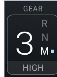
A visual signal may recommend shifting to a more optimal gear for fuel consumption. The signal appears above the display of the currently selected gear. The example below recommends that the driver shift up from 3rd gear to 5th.
