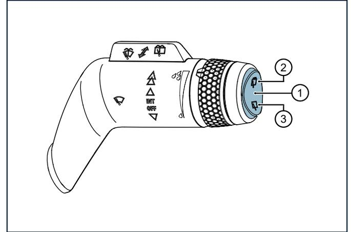
1. OFF - The top and bottom of the switch sit proud of the Stalk end. The rear wiper is off.
