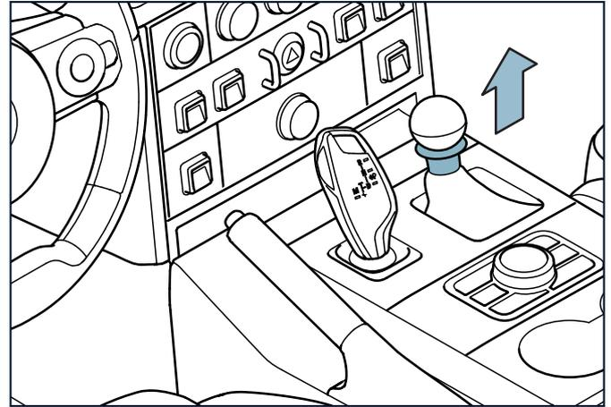
Always check that the transfer case selector is firmly engaged in one of the four positions before moving the gear selector from N (Neutral).
