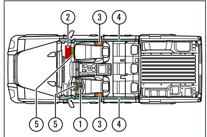
**Frontal air bags.** The driver's air bag (1) is in the steering wheel, and the front passenger's air bag (2) is above the glove compartment. These air bags deploy in front of the driver and front seat passenger to reduce the risk of injury to the head, neck, face, chest, and legs in severe frontal or near-frontal collisions.
