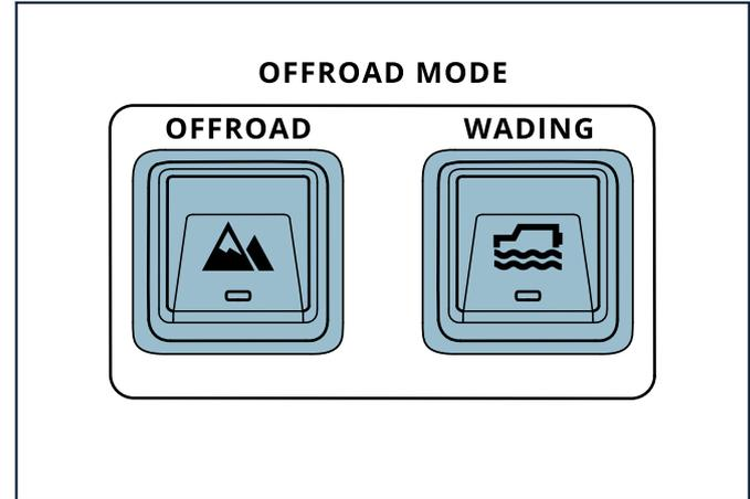
Release the button, then press it again within 15 seconds to confirm activation. An audible confirmation that Wading Mode is active will be heard, and the LED in the WADING button will turn on. Wading Mode
