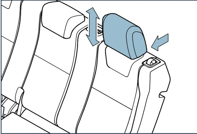
To adjust a head restraint, pull the head restraint upward until the desired height is achieved. To lower a head restraint, push the control button at the base of the head restraint, lower the restraint to the desired position, then release the control button to lock it
