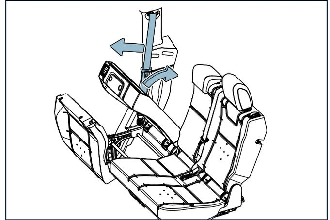
If the red indicator on the loop strap is visible, the seat back has not been locked. Occupants might be injured if your Grenadier is operated with unlocked, upright seat backs.
