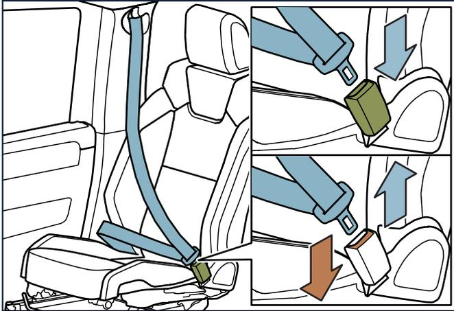
To fasten a seat belt in any of the four outboard seating positions (next to a front or rear door) around an adult occupant:
