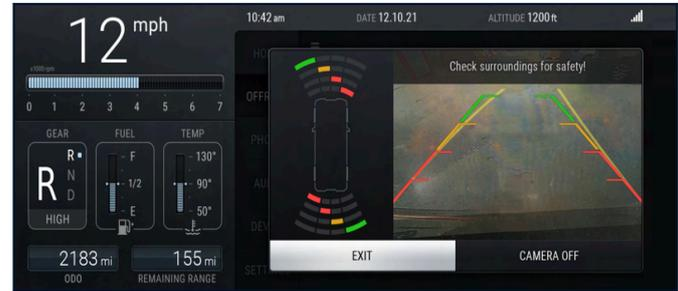
Parking Assist Rear sends sound and visual signals when you are backing close to an object at 10 mph (15 km/h) or less while moving backward.
