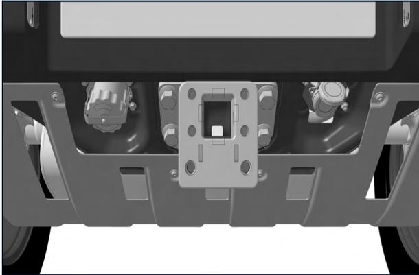
5. Insert the Removable Rear Winch into the 2" Receiver, ensuring the locking pin is correctly installed and secure with the R-Clip.
