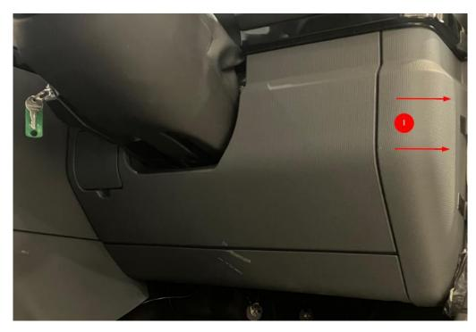
Step 2 Remove second cover by disassembling three screws (Torx TX20).
