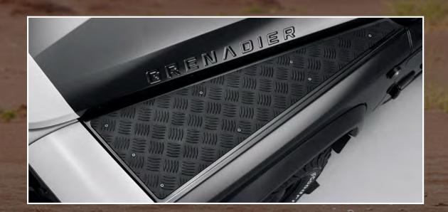
USMCA and Rest of World fenders can take a 90kg load without the checker plate e.g. sitting\* Additional fender reinforcement structure standard on USMCA and ROW vehicles.
